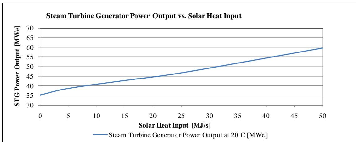
**Figure 5-1 Steam Turbine Generator Output vs. Solar Heat Input<sup>1</sup>**
